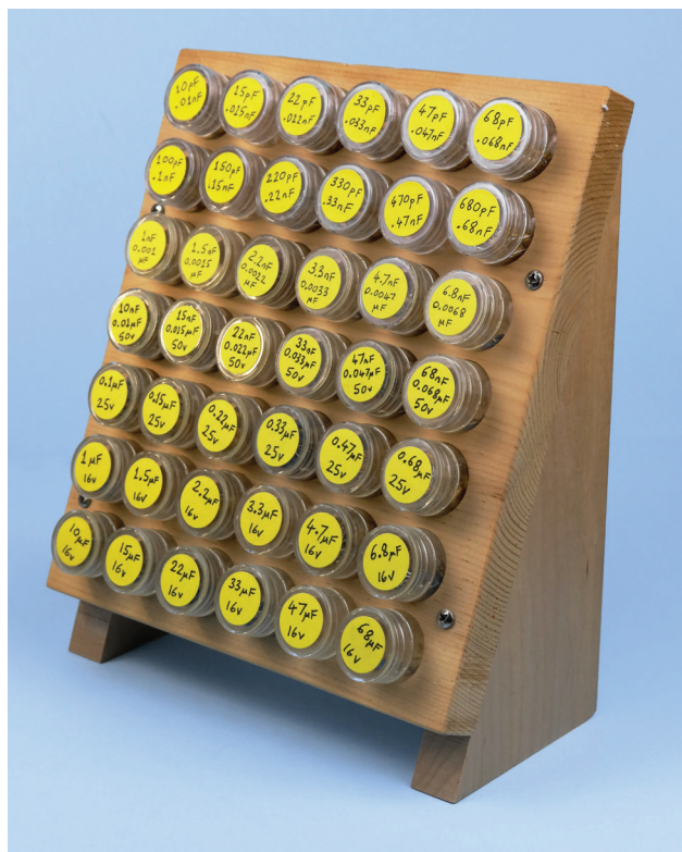
Figure 24-7. Desktop storage unit for containers of capacitors.
