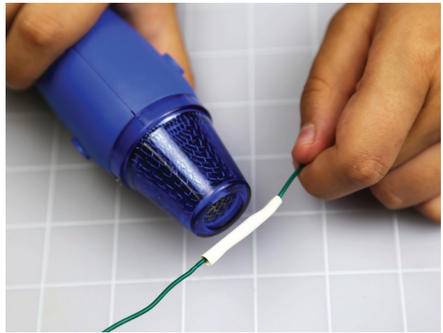
Figure 12-39. Preparing to insulate your solder joint.
