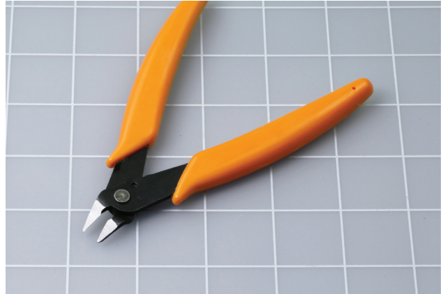
Figure 6-4. Flush cutters may reach into tinier spaces than wire cutters.
