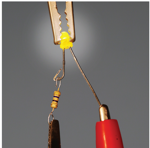
Figure 13-1. Ready to measure the heat tolerance of a 3mm yellow LED.
