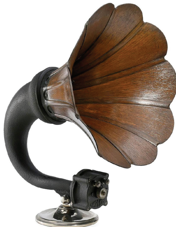
Figure 26-5. This beautiful Amplion horn illustrates the efforts of early designers to maximize efficiency in an era when the power of audio amplifiers was very limited.
