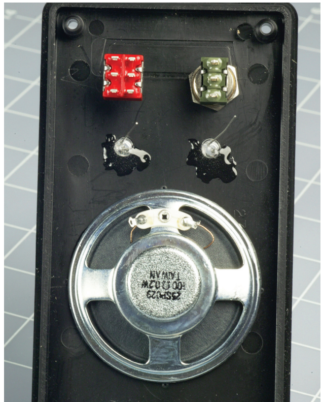
Figure 17-25. Mounting components under the lid of the box.
