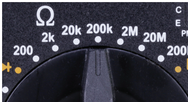
Figure 1-23. A manual meter requires you to select the range
