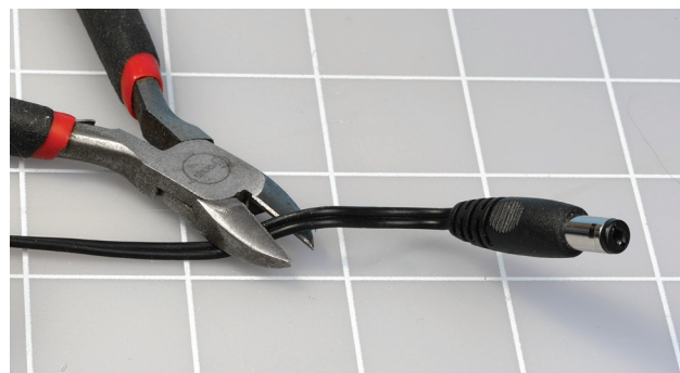
Figure 12-42. Trimming the wire from the AC adapter must be done when the adapter is not plugged into the wall.
