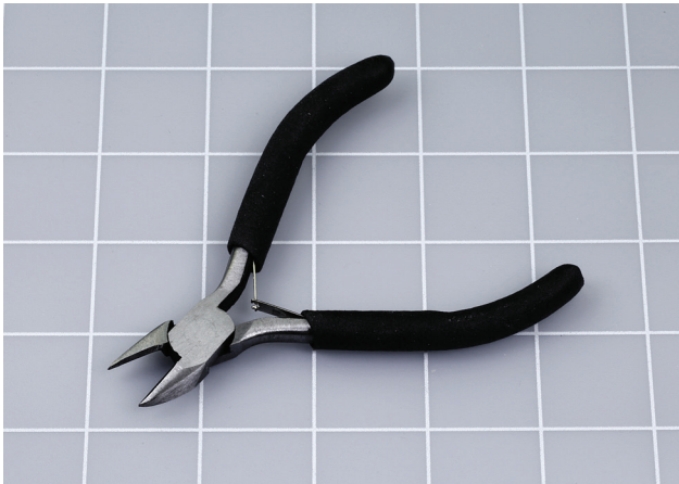
Figure 6-3. Wire cutters should be no more than five inches long.
