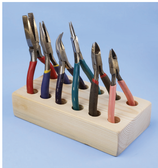
Figure 24-11. A 7" piece of two-by-four is all you need to store pliers and wire cutters accessibly.
