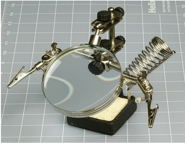
Figure 12-4. This version of the “helping hand” includes a wire spiral in which to park your soldering iron, a sponge to clean the tip, and a large magnifying glass.
