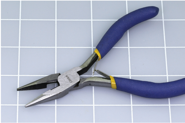
Figure 6-2. Appropriate pliers for electronics work should be no more than 5" long.
