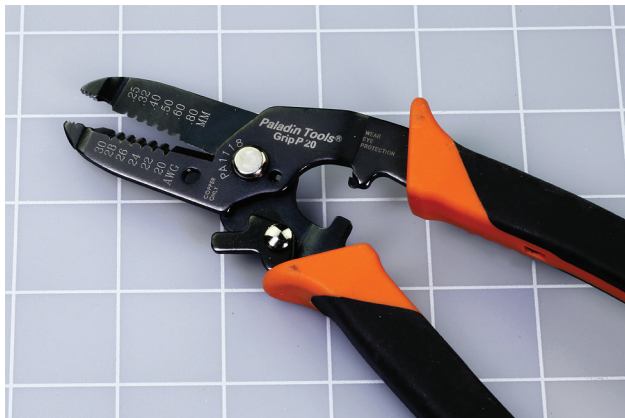
Figure 6-6. Wire strippers for removing insulation from wire.
