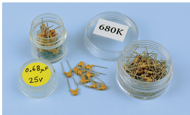
Figure 24-6. Trimmed resistors will fit in containers about 1-1/2" in diameter, while ceramic capacitors can be stored in similar containers 1" in diameter.
