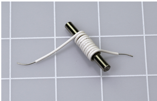
Figure 25-1. Just ten turns of wire can be sufficient to create a small electrical potential when a magnet moves through them.
