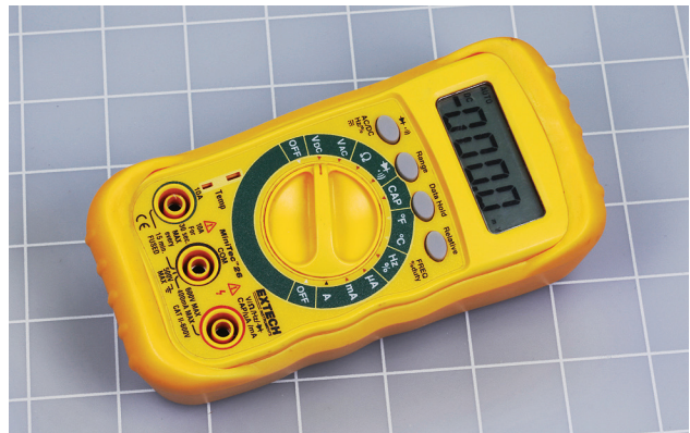
Figure 1-2. An auto-ranging meter.
