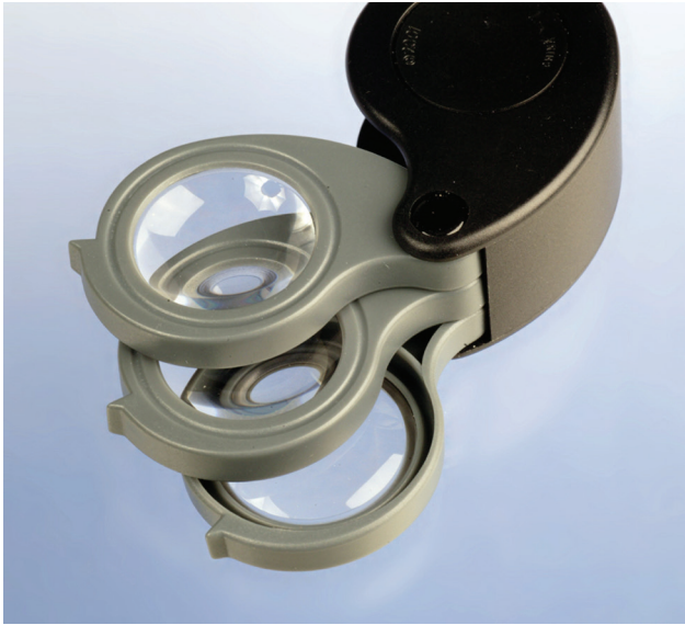
Figure 12-10. These three lenses are identical, but if you put two or three of them together, you multiply the total magnification.
