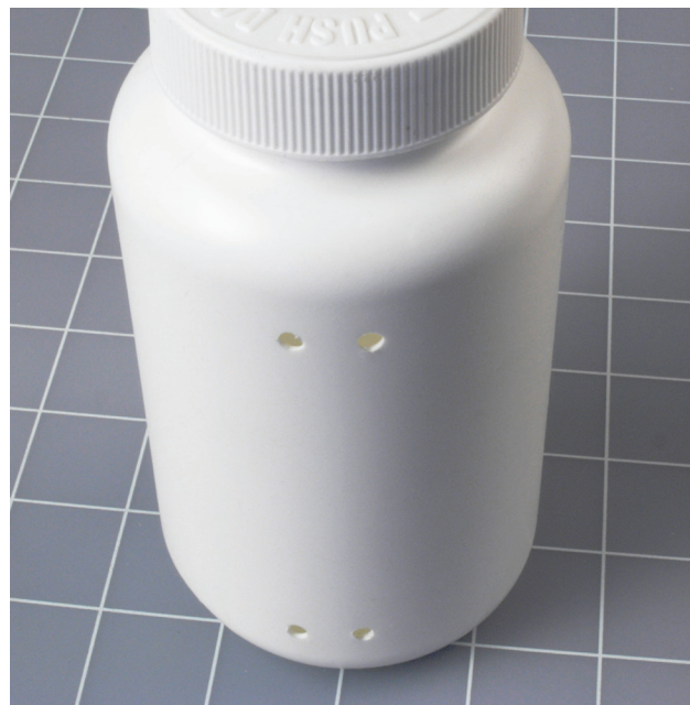
Figure 28-1. A suitable bottle for your coil. The holes will be used to anchor the wire.
