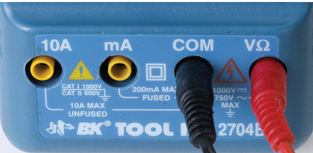
Figure 1-19. Where to plug in the meter leads.
