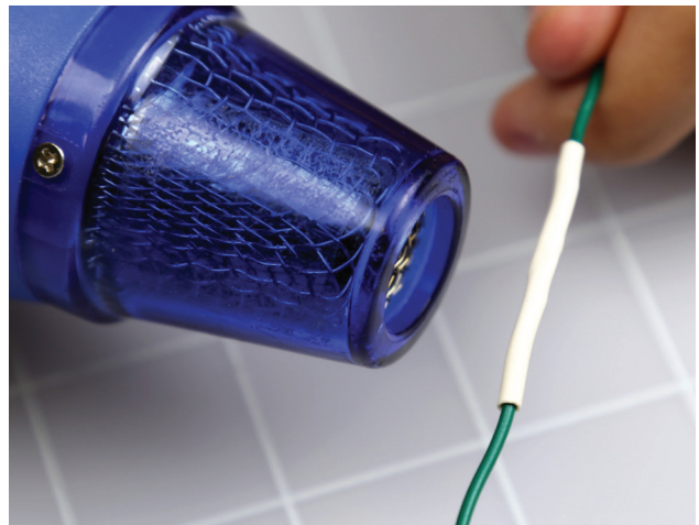
Figure 12-40. The heat-shrink tubing has shrunk, and the job is done.
