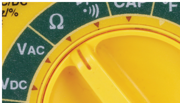
Figure 1-22. Selecting resistance in an auto-ranging meter.
