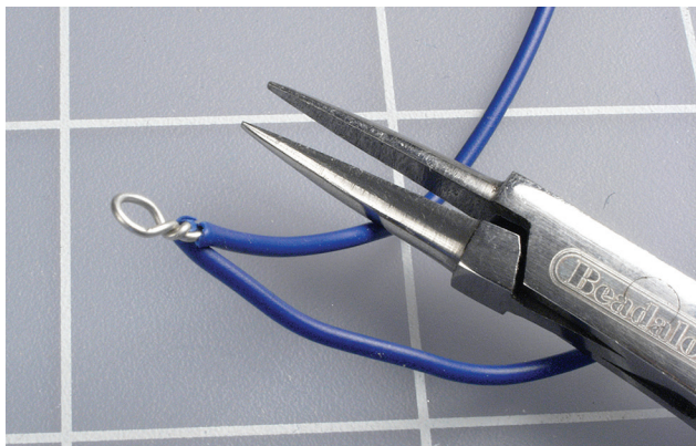
Figure 28-4. Create a loop in the section of wire that you exposed.
