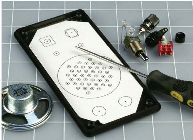
Figure 17-18. A layout for switches and LEDs under the box lid.
