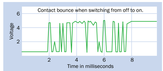
Figure 22-1. Fluctuations created by vibrating contacts when a switch is closed. (Derived from a datasheet at Maxim Integrated corporation.)
