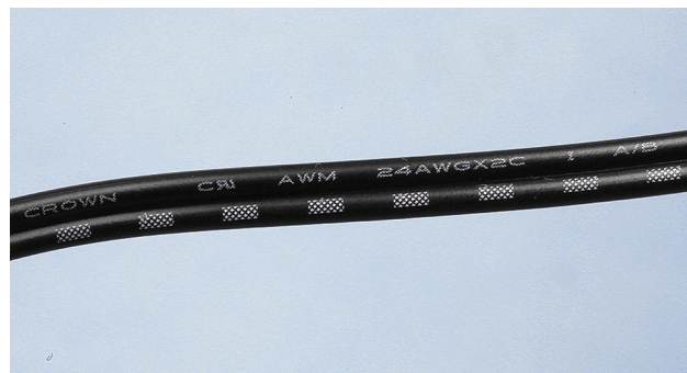
Figure 12-43. One conductor from your AC adapter may be marked, usually indicating that it is positive, but you need to make sure.
