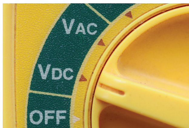
Figure 3-4. Setting an auto-ranging meter to measure volts.
